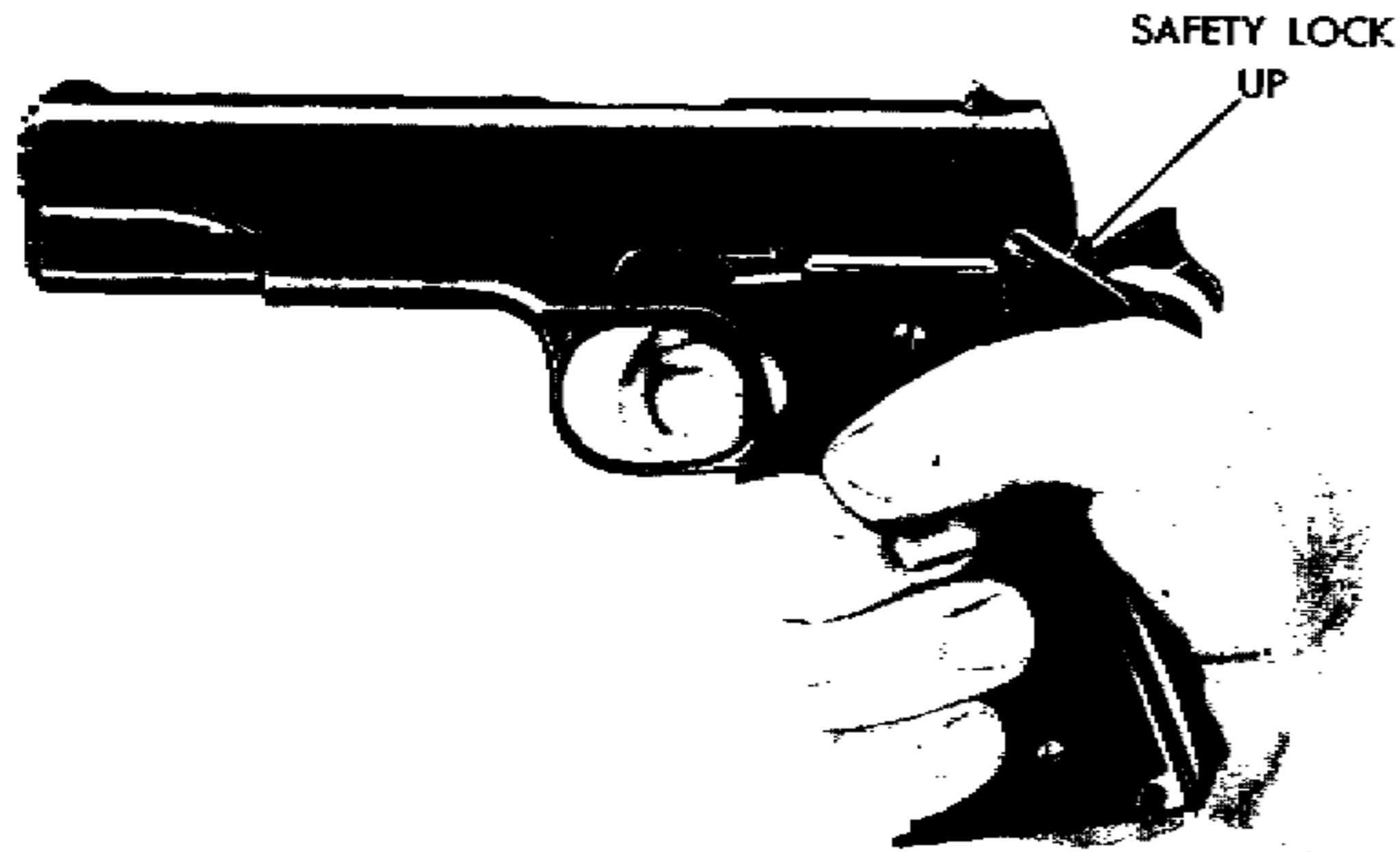
Figure 27. — Pistol M1911A1, Hammer Back, Safety Lock Upward in Safety Position, Hand Grasping Stock So Grip Safety Is Depressed, Finger Squeezing Trigger
