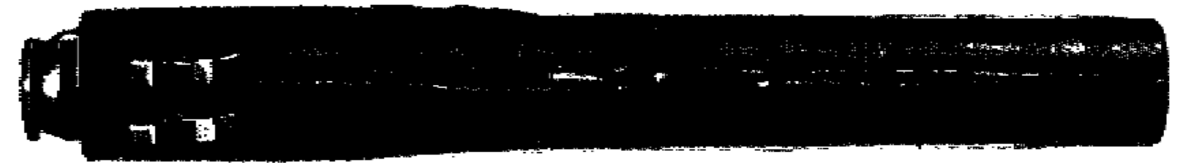
Figure 69. Damage caused by firing with bullet lodged in bore, cal..45 automatic pistol M1911.
